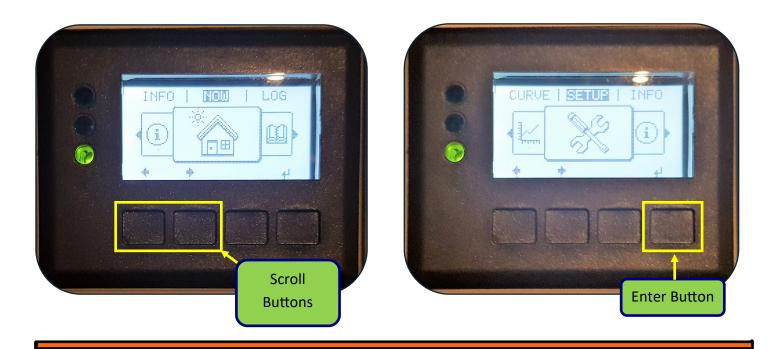
Press the **Scroll Down** button until you arrive at **WiFi Access Point**. Press the **Enter** button. Press the **Enter** button again to **Activate WiFi Ap**.
